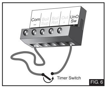
COMBUSTION AIR OR ALARM CONTACT
